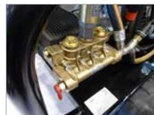
SOUPAPE THERMOSTATIQUE POUR PROTÉGER LA POMPE CONTRE LES SURCHAUFFES POSSIBLES
